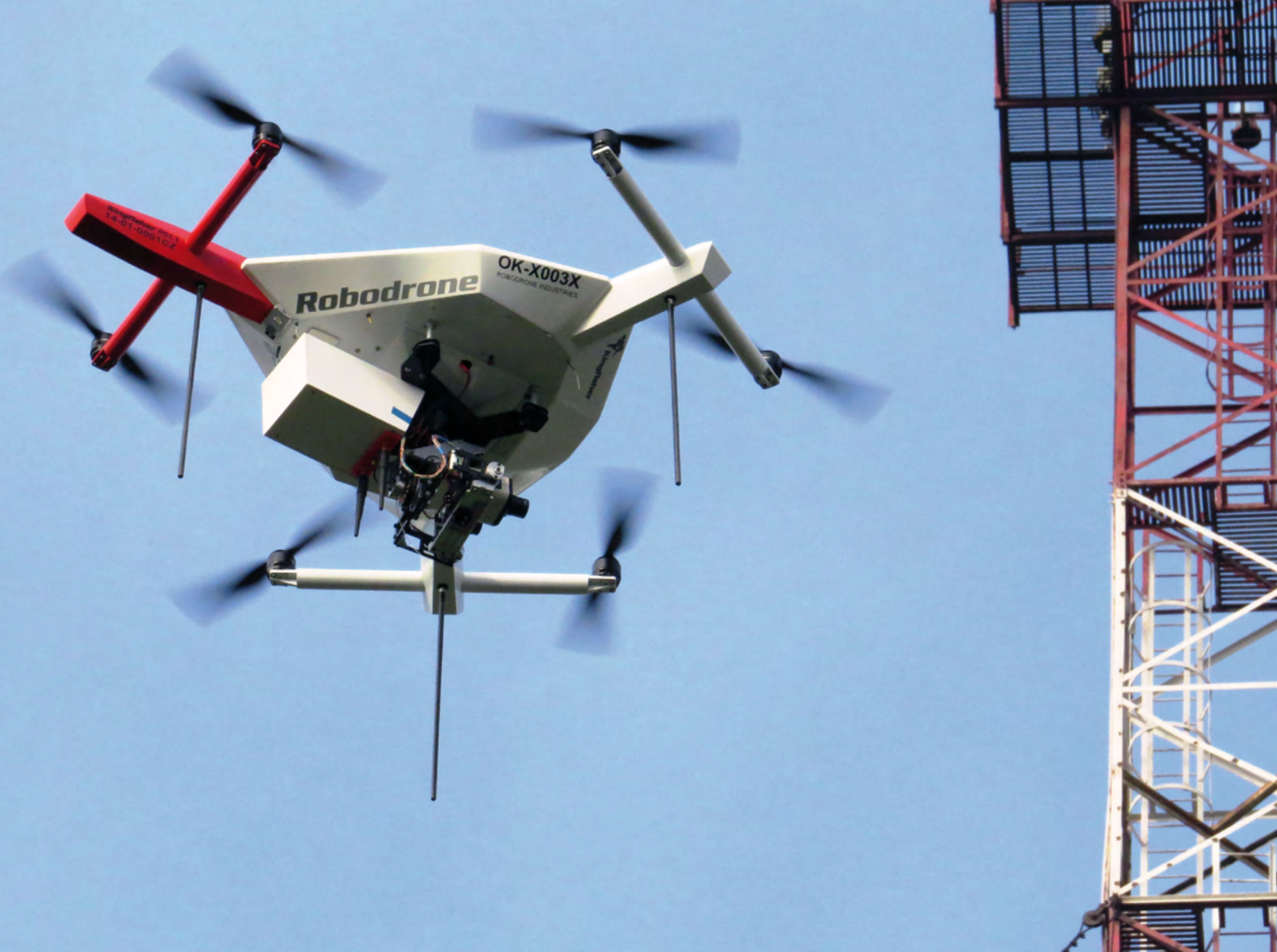
Dron s termokamerou při testovacím letu na OBS Tušimice. A drone with a thermal imaging camera during a test flight at the Tušimice Observatory.
